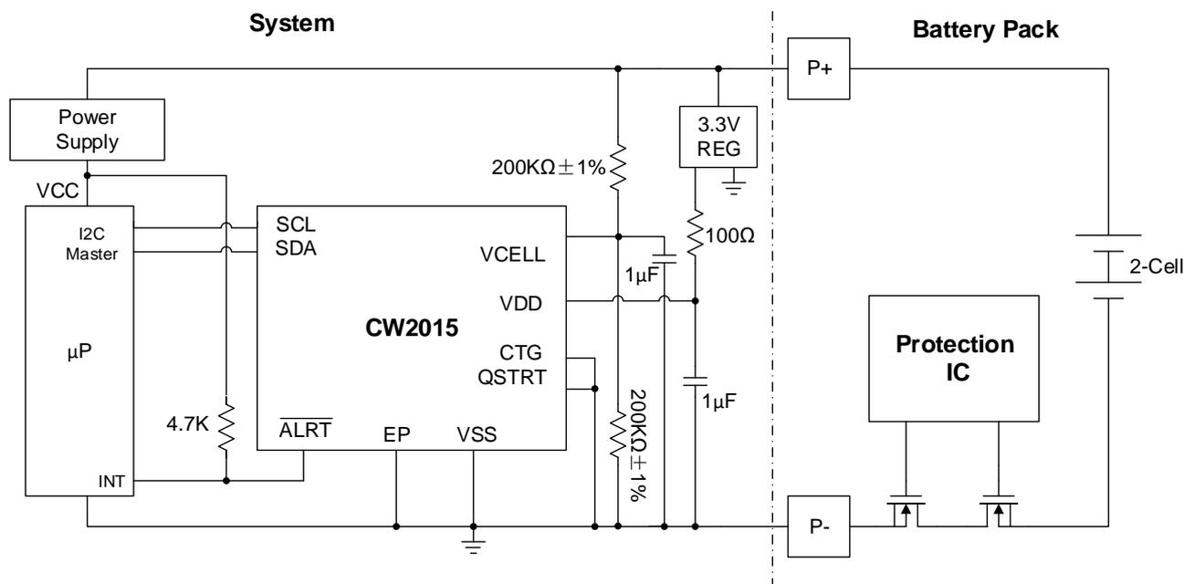
Figure 10. Typical Application for 2-Cell and System Side
