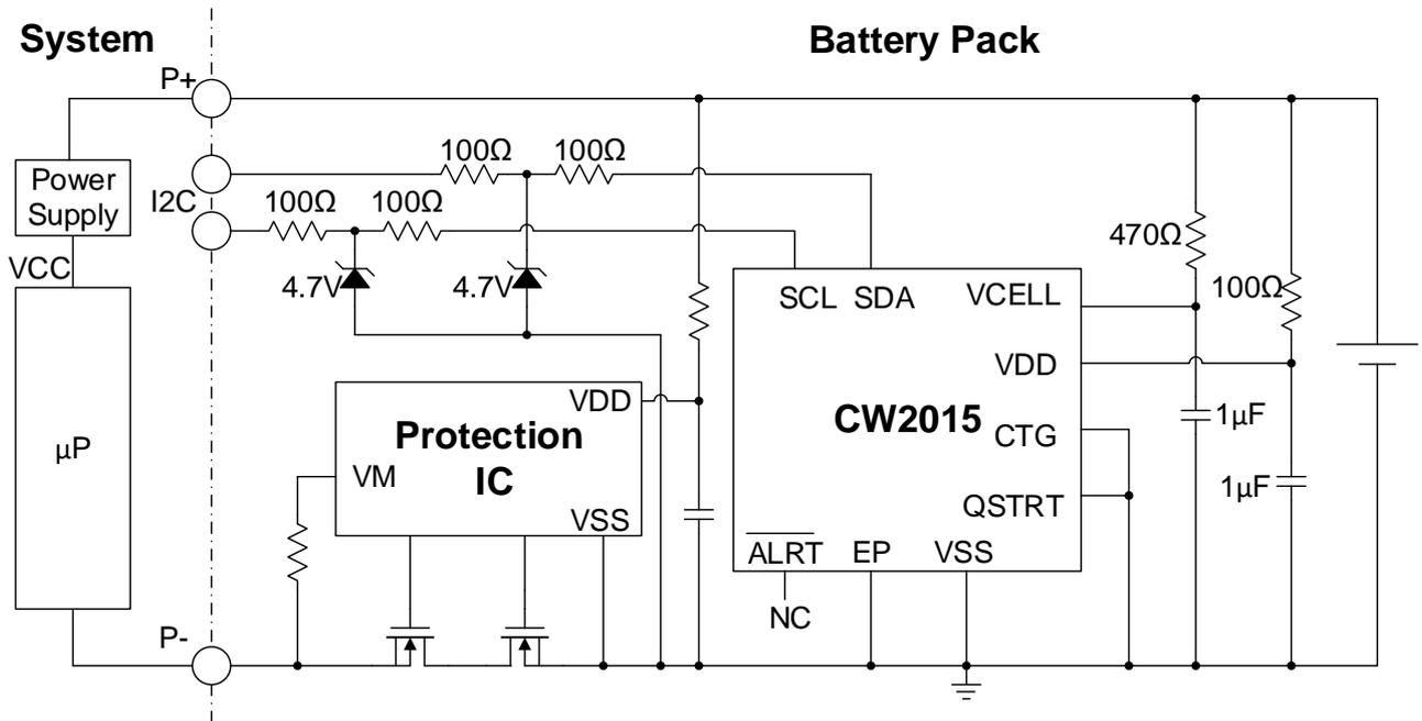
Figure 2. Typical Application for 1-Cell and Pack Side
