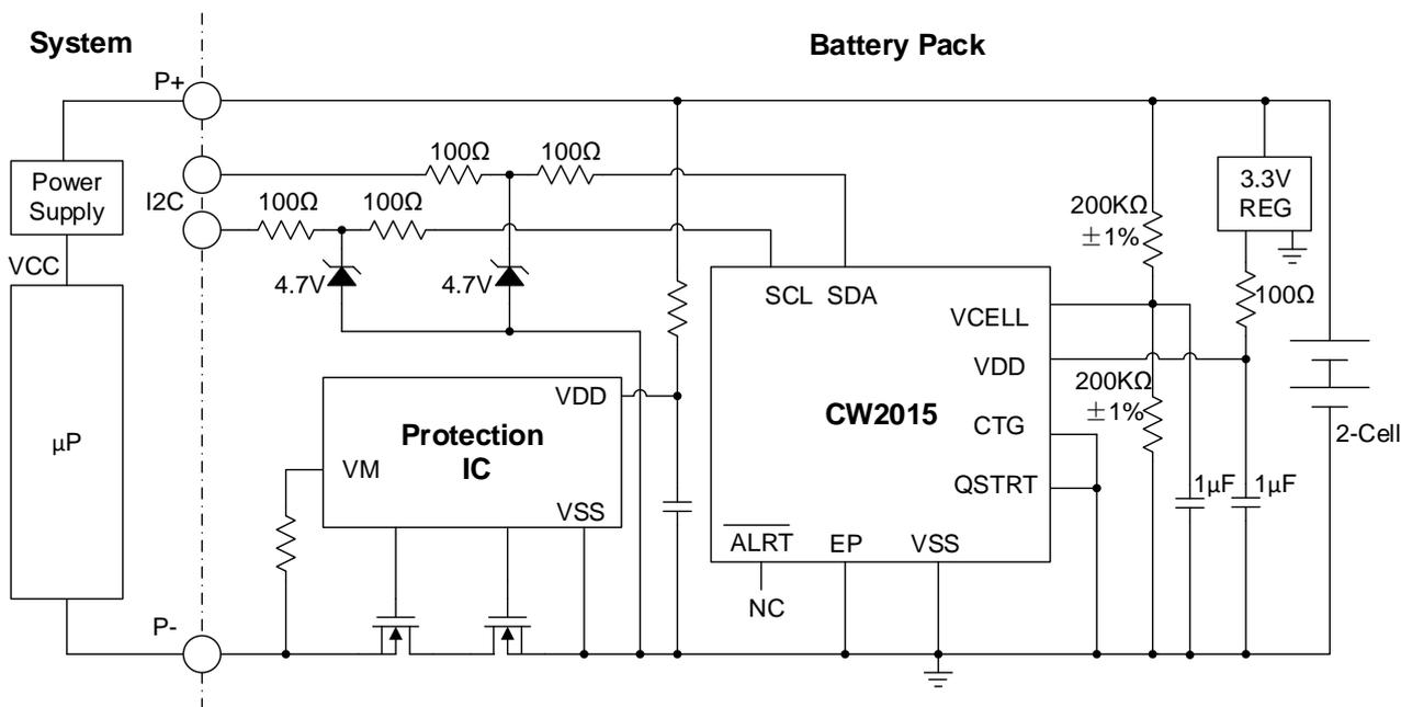
Figure 11. Typical Application for 2-Cell and Pack side
