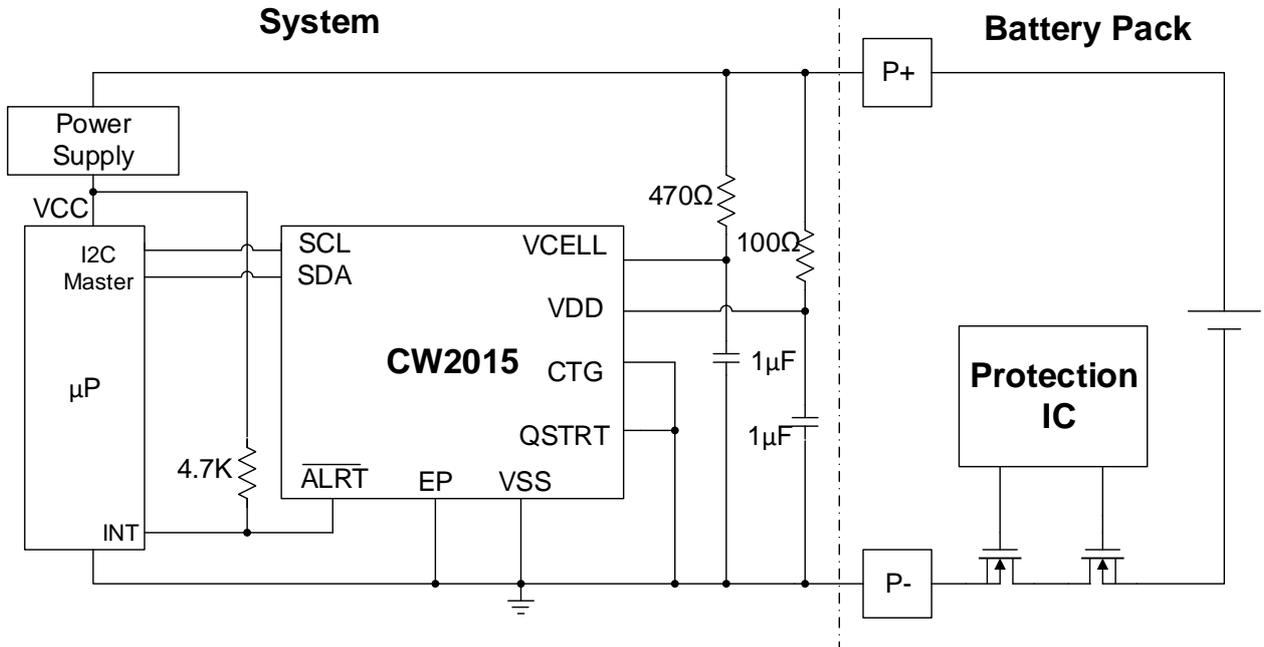
Figure 1. Typical Application for 1-Cell and System Side
